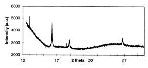
b) The presence of a second phase can be inferred from the sharp peaks observed in fig. 1 at 12.94" and 18.34". These peaks have been indexed as the 110 and 200 peaks of a bcc structure with a lattice constant 2% larger than the fcc Pd one. Very faint 211, 220 and 310 peaks, hardly distinguishble from the noise, have been also detected.
