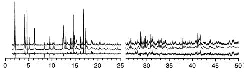
Observed (top), calculated (middle) and difference (bottom) profiles for the present state of the refinement of ITQ-l(P). The second half of the profile has been scaled up by a factor of 5 to show more detail.
