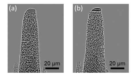
Figure 1 – Projection obtained on the beamline for the same sample (a) in pristine state and (b) after an ex-situ redox cycle.
