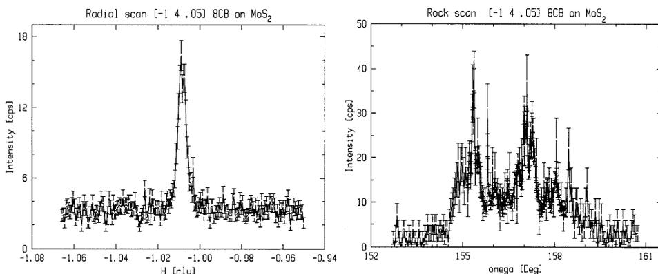
**Figure 1:** Radial and rock scans of the  $[-1\ 4\ \epsilon]$  peak of 8CB on  $\text{MoS}_2$ . The full width at half maximum of the radial scan, equal to  $0.075^\circ$ , is determined by the Q resolution but the rocking curve is very large.
