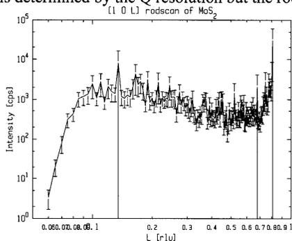
**Figure 2:** Example of  $[1\ 0\ L]$  rodscan of  $\text{MoS}_2$ . The Vineyard peak is smeared out by the sample roughness but the intensity is quite high all along the rod upto the  $[1\ 0\ 1]$  Bragg peak. Scan done with a 0.4 mm Al attenuator (attenuation factor of 120 at 8.2 KeV)
