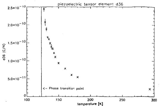
Figure 4: The  $d_{36}$  piezoelectric constant as function of temperature.
