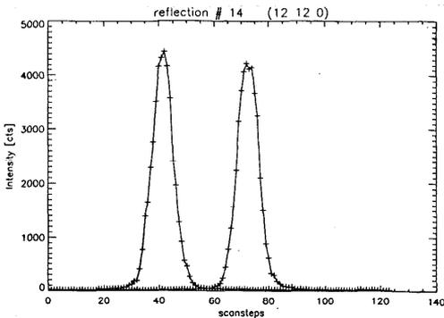
Figure 3: Separation of the  $(12\ 12\ 0)$  peak at 129K in the presence of an electric field.
