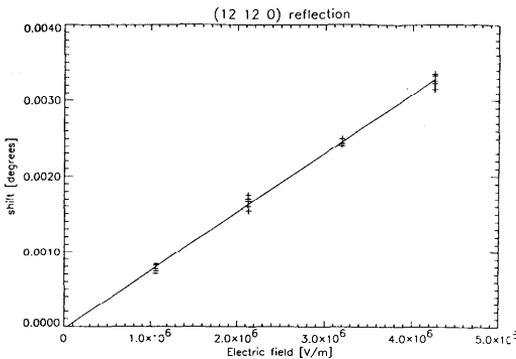
Figure 1: The shift as function of the applied electric field as measured for the  $(12\ 12\ 0)$  reflection.
