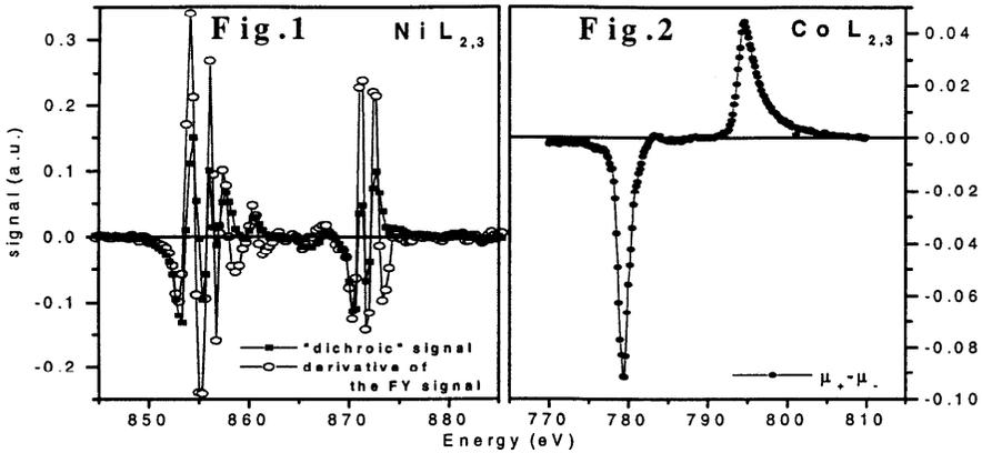
Despite this, the Co FY was successfully measured, but as it will be seen later, the dichroic signal could not be worked out properly. The zero-thickness limit was used for the 20Å Co layer ( $I_{FY} \sim \mu$ ), while for the 200Å film the dependence is no more linear: in this last case, 2 measurements at different angles were performed in order to deduce  $\mu$ .
