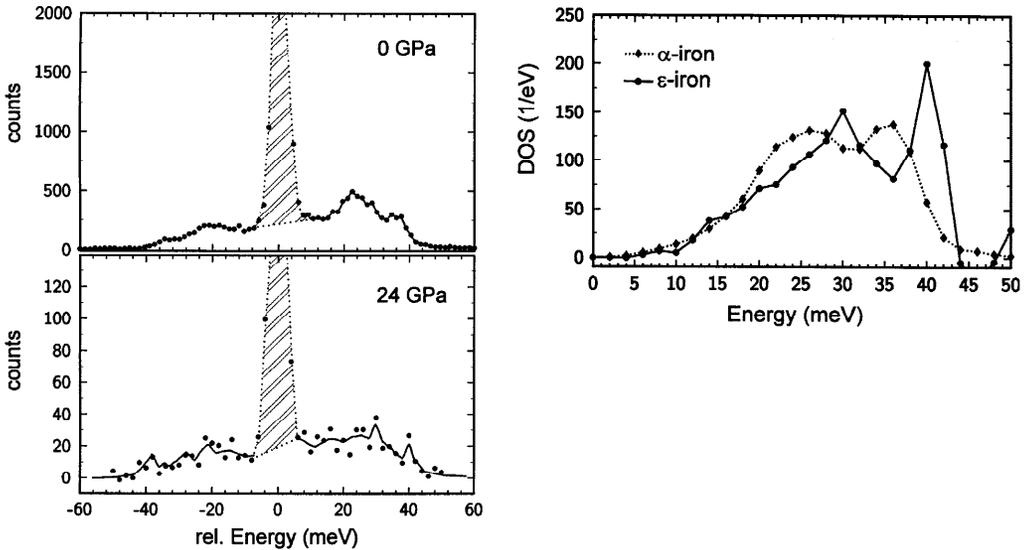
**Fig. 1.** (left panel) Inelastic nuclear scattering of iron at ambient pressure and at 24 GPa, corrected for background. (right panel) Derived Phonon DOS for both iron modifications.
