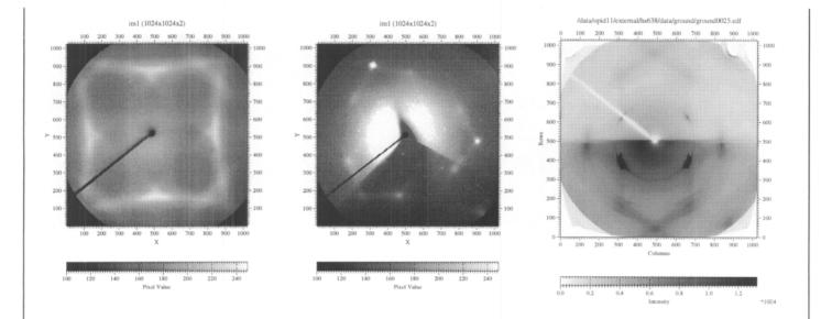
Fig. 1: Diffraction patterns (*Frelon* area detector) of hardness impressions in (100)-Si (a), (111)-Ge (b), and a ground Si (c) surface. No polycrystalline material was found except some debris of Si-I structure on the ground surface.
