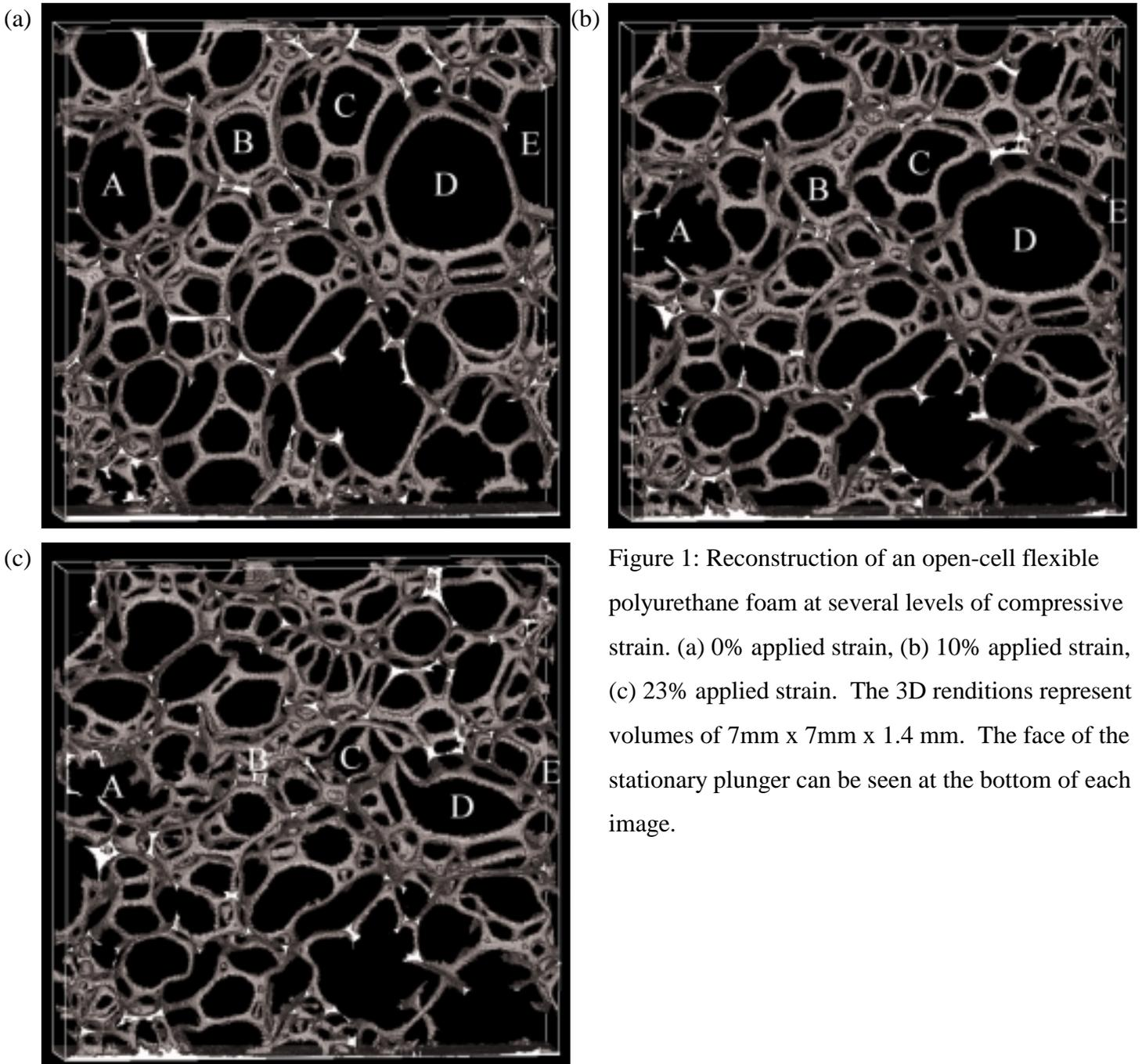
Figure 1: Reconstruction of an open-cell flexible polyurethane foam at several levels of compressive strain. (a) 0% applied strain, (b) 10% applied strain, (c) 23% applied strain. The 3D renditions represent volumes of 7mm x 7mm x 1.4 mm. The face of the stationary plunger can be seen at the bottom of each image.
