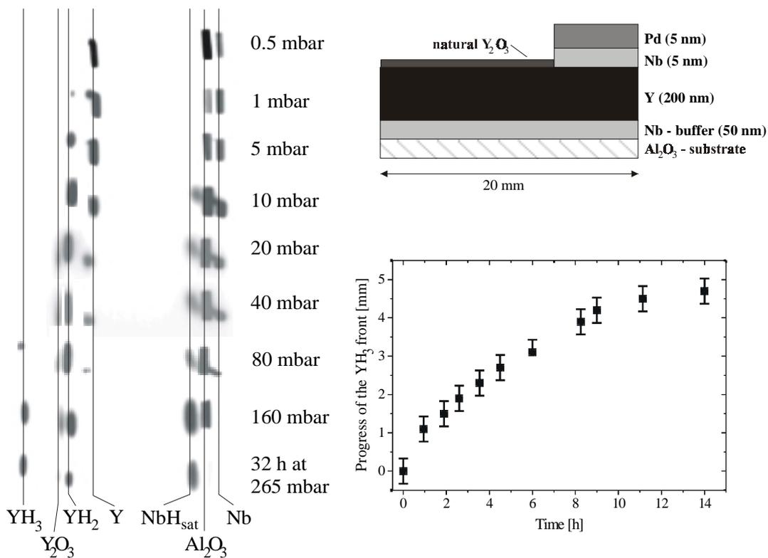
*Series of topographies visualizing H- diffusion within the 200 nm thick Y film at  $250^\circ\text{C}$  (left). The progress of the diffusion front is depicted below the sample architecture (right).*
