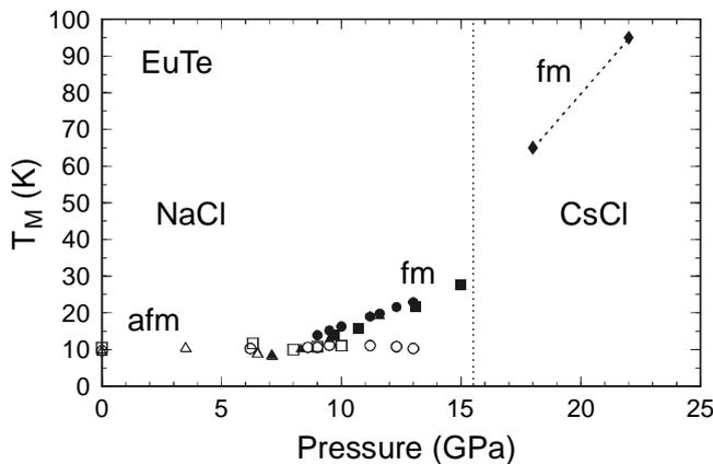
**Fig. 2:** Magnetic phase diagram of EuTe. The open symbols exhibit the antiferromagnetic Neel-temperature  $T_N$  and the closed symbols the ferromagnetic Curie-temperature  $T_C$ . The vertical dashed line indicates the middle of the (broad) NaCl - CsCl phase transition at about 16 GPa [7]; deduced from: ME ( $\circ$ ,  $\bullet$ ) [6], neutron diffraction ( $\square$ ,  $\blacksquare$ ) and present NFS study ( $\blacklozenge$ ).
