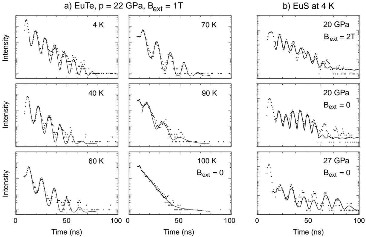
**Fig. 1:** (a) Eu-151 NFS spectra of CsCl-phase EuTe at 22 GPa and various temperatures with an external field of 1T applied parallel to the synchrotron beam. The ferromagnetic ordering temperature is amount to 95 K.(b) Magnetic NFS spectra of NaCl-phase EuS at 20 GPa and of CsCl-phase EuS at 27 GPa. The solid lines are fits adopting the dynamical theory of nuclear resonance scattering.
