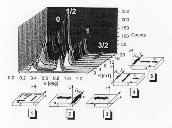
Fig. 1. Time differential SMR curves taken on a MgO(001)/[57Fe(25 Å)/Cr(14 Å)]<sub>20</sub> superlattice in increasing magnetic field. The appearance of the antiferromagnetic reflections shows the rotation of the layer magnetisations at the bulk spin flop transition. The system of coordinates is fixed to the superlattice.
