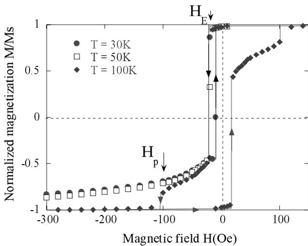
Figure 1: Magnetization versus applied field for three different temperatures on  $Gd_{40}Fe_{60}(1000 \text{ \AA})/Tb_{55}Fe_{45}(30 \text{ \AA})$ .
