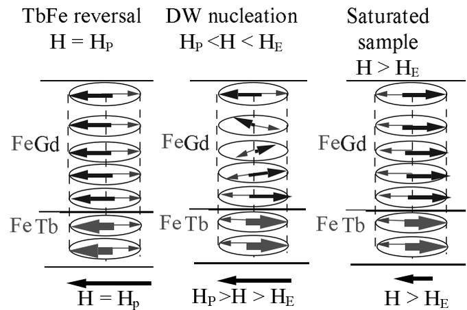
Figure 2: Magnetic configuration in  $GdFe/TbFe$  bilayer for different applied field
