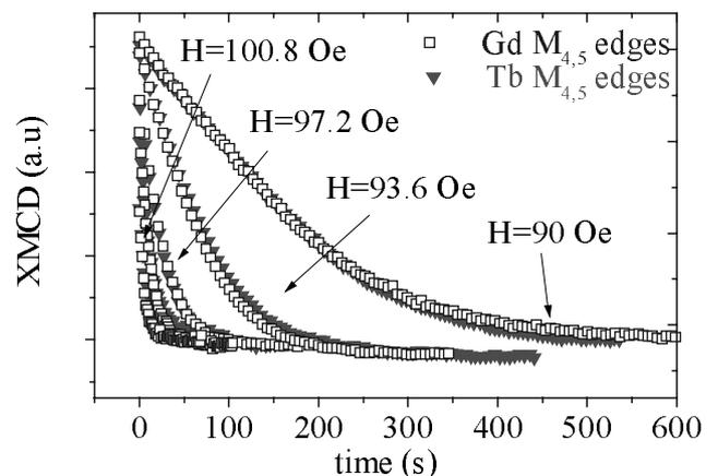
Figure 4: XMCD after effect measurements for different field: XMCD signal at the  $Gd$ , and  $Tb M_{4,5}$  edges as a function of time
