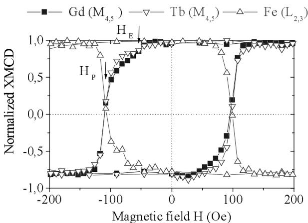
Figure 3: XMCD signal at the  $Fe L_{2,3}$  edges and the  $Gd$ , and  $Tb M_{4,5}$  edges as a function of the applied field at 100K on  $Gd_{40}Fe_{60}(1000 \text{ \AA})/Tb_{55}Fe_{45}(30 \text{ \AA})$ .
