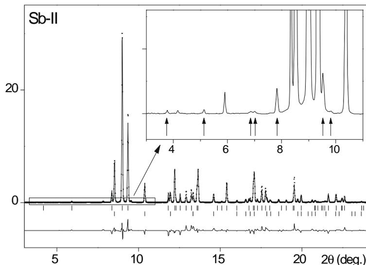
**Figure1.** Rietveld fit to the host-guest structure of Sb-II at 10.3GPa. Some of the low-angle additional reflections not accounted for by this structure are indicated in the inset.
