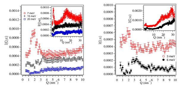
Figure 1. Dynamic structure factor in the Brillouin region at different energies. a)  $Li_2O-2B_2O_3$  and b)CKN. The inset shows the full experimental Q-range. The spectra have been shifted vertically for clarity.
