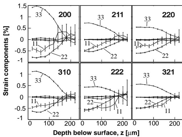
Fig. 1: Depth dependent strain tensor components of a shot peened Timetal sample. The error bars represent  $\pm 2$  standard deviations. The large errors for the 11 component result from the restricted sample rotation of only  $\pm 30^\circ$  around the surface normal.
