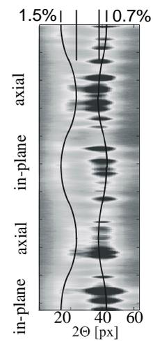
Fig. 2:  $\alpha\{102\}$  (left) and  $\beta\{200\}$  (right) diffraction rings in polar coordinates indicating epitaxial growth and micro strain.
