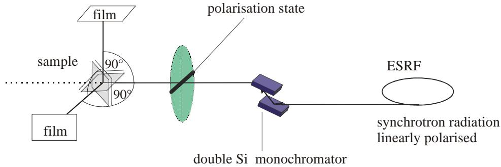
Figure 3: experimental arrangement
