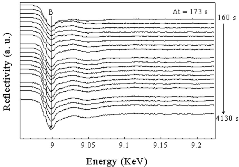
Fig. 1. Reflectivity spectra measured during the oxygenation process
