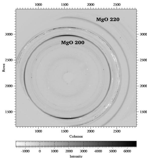
Figure 3: Diffraction pattern for MgO at 8 GPa. Background from the amorphous boron was subtracted.
