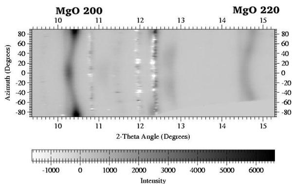
Figure 4: Cake file showing the variation of the d-spacings and intensities as a function of the azimuth angle (between  $-90$  and  $90^\circ$ ) for MgO at 8 GPa.
