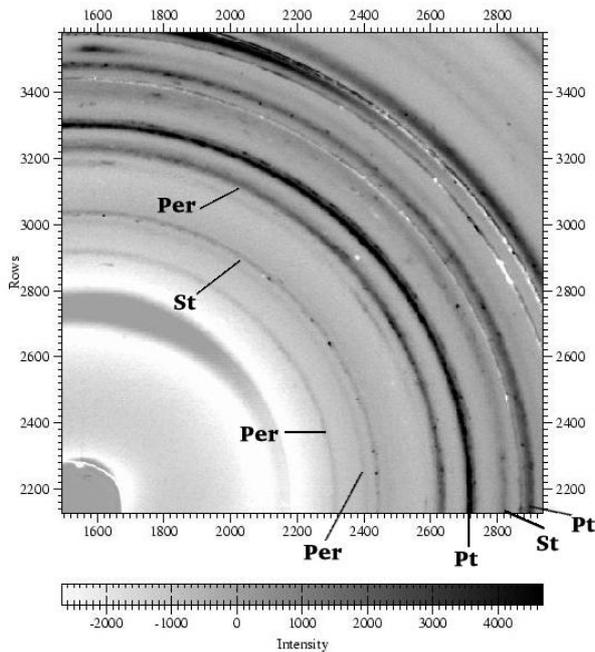
Figure 1: Diffraction pattern for perovskite experiment at  $P = 25$  GPa. Peaks from perovskite, stishovite and platinum are shown. Background from amorphous boron was subtracted for this pattern.
