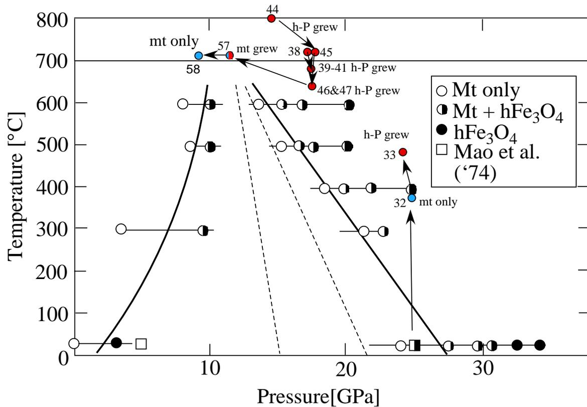
Figure 1. Results from experiment HS-1214 plotted in terms of the pressure-temperature conditions of particular diffraction patterns (numbered coloured symbols; blue/light grey is magnetite only and red/dark grey symbols indicate the presence of both the high-P phase and magnetite). Arrows indicate the sequence of the diffraction patterns. Other black and white symbols and proposed phase boundaries are from Huang & Bassett (1986) and Mao et al. (1974).
