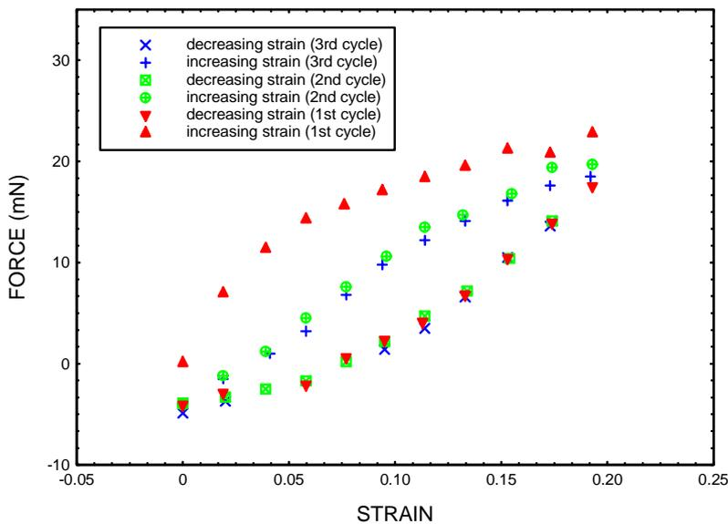
**Figure 1:** A force / strain plot for a triple-cycle deformation experiment illustrating the hysteresis characteristics of the foam strut.
