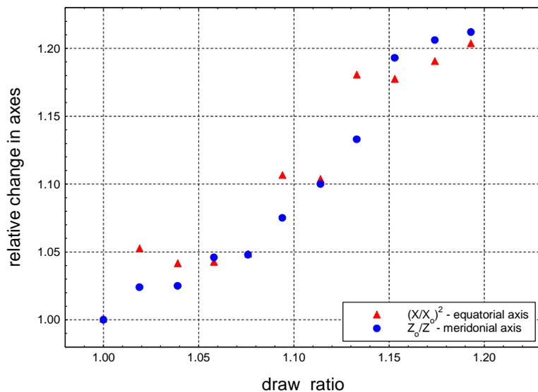
**Figure 2:** Plot from the analysis of SAXS pattern ellipse shape variation during deformation up to a strain of about 0.2. The approximately linear relationship between the draw ratio and the relative change in major and minor axes suggests that the deformation, within this strain range, is affine in manner.
