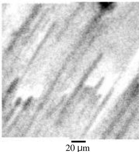
Figure 1. Silicon fluorescent yield mapping of a montmorillonite (Swy-2) clay gel at 50 g/l (resolution : 1  $\mu\text{m}$ , dwell time : 400 msec).
