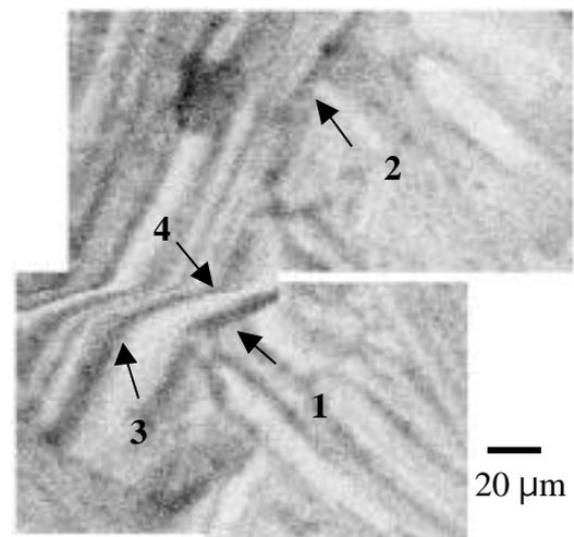
Figure 2. Silicon fluorescent yield mapping of a montmorillonite (Swy-2) clay gel at 50 g/l (resolution : 1  $\mu\text{m}$ , dwell time : 400 msec). The arrows show the various types of orientational defects.
