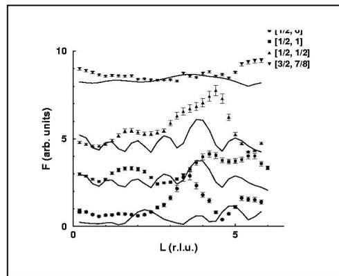
Fig. 1. Experimental and simulated fractional order rods of the Ge(111)-c(2x8) surface reconstruction.
