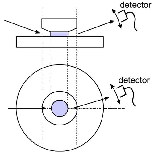
**Fig. 2** Schematic of the scattering geometry. Top and bottom panels show the scattering directions perpendicular and parallel to the plane of the confining surfaces. The dark area represents the colloidal suspension.
