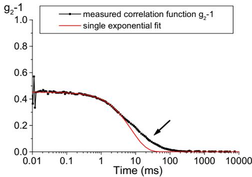
**Fig. 3** Time correlation function  $g_2(t)$  measured on a solution of 7 wt% 210 nm diameter silica spheres in a 3cP water/glycerol mixture at a gap width of ca. 700 nm. The momentum transfer was  $q_{\parallel} = 5.8 \cdot 10^{-3} \text{ nm}^{-1}$ . Fitted to the first part of the correlation function is a single exponential decay. The deviation from the single exponent (indicated by arrow) cannot be fitted by an exponential decay and is probably an effect of the confinement.
