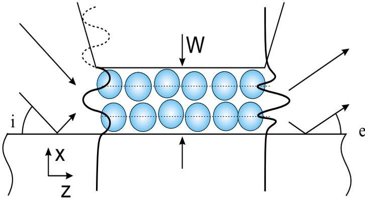
**Fig. 1** Schematic drawing of the waveguide setup. The transversely coherent x rays are incident from the side at a grazing angle and propagate between the confining surfaces. The motion of the colloidal particles will result in a fluctuating speckled far field diffraction pattern behind the exit of the waveguide.
