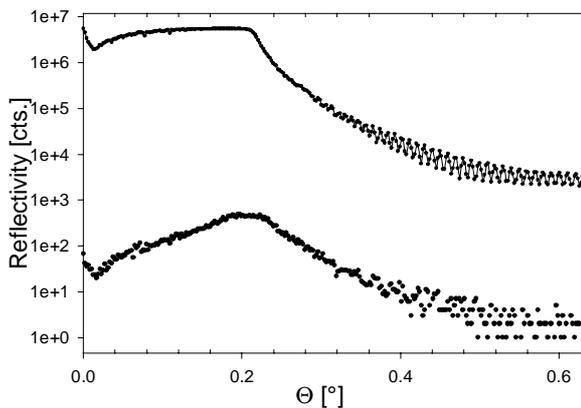
Fig. 2. From the period of Kiessig beats [3] of the electronic reflectivity the thickness of the iron layer can be estimated (upper curve). The nuclear reflectivity shows its maximum at the critical angle of the total reflection at 3.8 mrad. The iron sample was measured at a smaller angle (1.66 mrad =  $0.095^\circ$ ) where the penetration depth in iron is about 3 nm.
