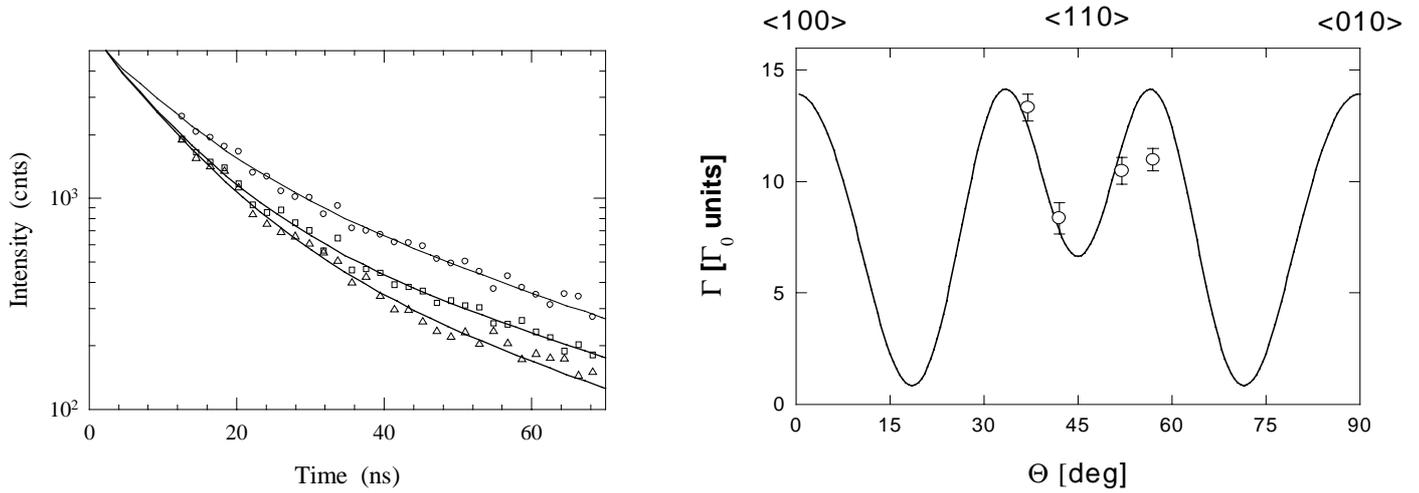
Fig. 1. (left) Intensity decay of the nuclear resonant scattered quanta from iron measured at different temperatures and at the same grazing angle of 1.66 mrad. Temperatures 1090K (circles), 1200K (squares) and 1230K (triangles); (right) intensity decay acceleration  $\Gamma$  at 1200K from the near-surface iron layer as a function of the azimuth angle between the SR direction and the (100) iron crystal axis.
