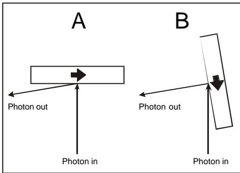
Experimental geometry: the sample is magnetized in-plane
