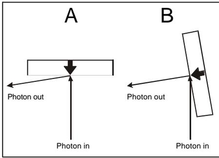
Experimental geometry: the sample is magnetized out-of-plane
