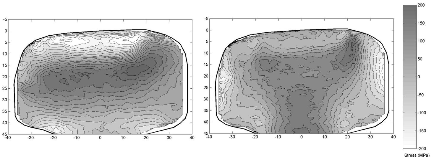
*\*Figure 1. High resolution transverse (left) and vertical (right) residual stress maps of the head of a 4 mm thick heavily worn US rail section [Scan matrix 1-2 mm, gauge 0.5 mm square, 6000 data points at ~10 seconds per point]*
