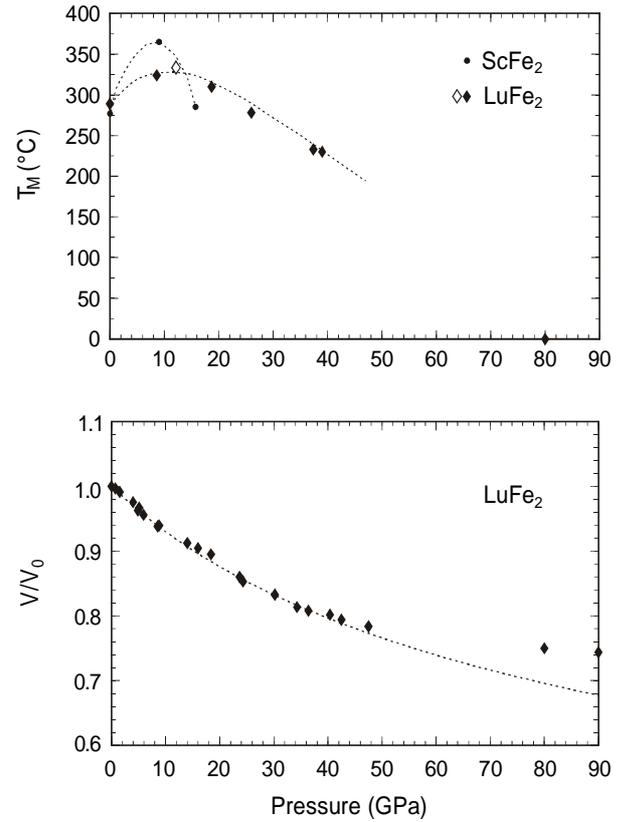
Fig. 2: top: magnetic ordering temperatures at various pressures. bottom: pressure - volume dependence of LuFe<sub>2</sub>
