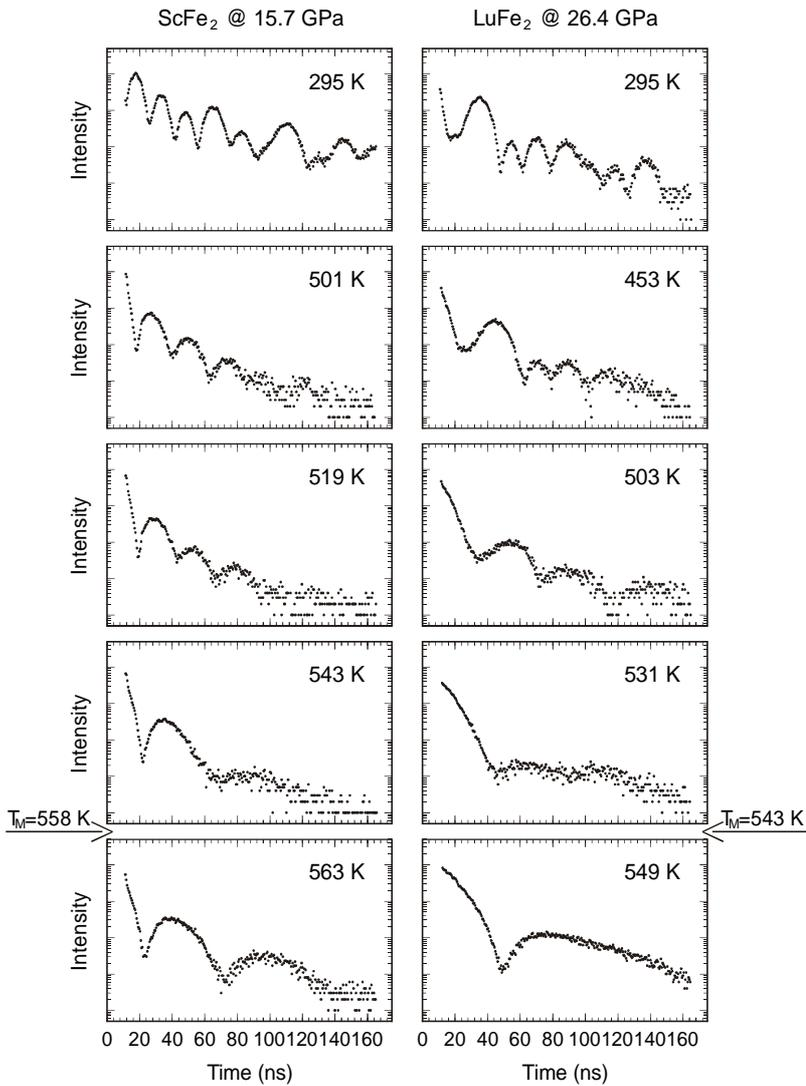
Fig. 1: Temperature dependent NFS Spectra of ScFe<sub>2</sub> at 16 GPa and LuFe<sub>2</sub> at 26 GPa. The arrows denote the magnetic ordering temperature.
