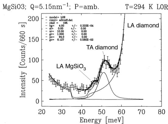
As shown in this figure, the acoustic longitudinal excitation from the sample is almost at the same energy as the signal related to the transverse acoustic phonon of the diamond anvil. The diamond window is indeed characterized by very high acoustic velocities, which makes any analysis impossible at high-pressure in the geometry we had during the experiment.
