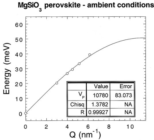
Assuming a sine function for the dispersion of this longitudinal acoustic mode, we obtain a mean longitudinal acoustic velocity  $V_p$  of  $10780 \pm 83 \text{ ms}^{-1}$ , which is in good agreement with the value of  $10940 \text{ ms}^{-1}$  determined by Brillouin spectroscopy [1].
