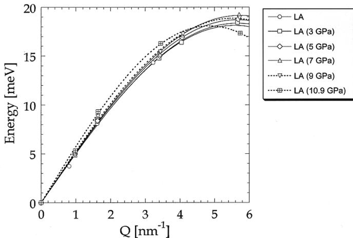
In addition to sound velocities determination as a function of pressure, the preliminary results presented below might indicate that such a transition indeed proceeds via a softening of the longitudinal branch along  $\zeta 00$ , which starts at 9 GPa and is clear at 10.9 GPa close to the edge of the first Brillouin zone. However, complementary experiments on other crystal orientations are needed to strengthen such conclusions.
