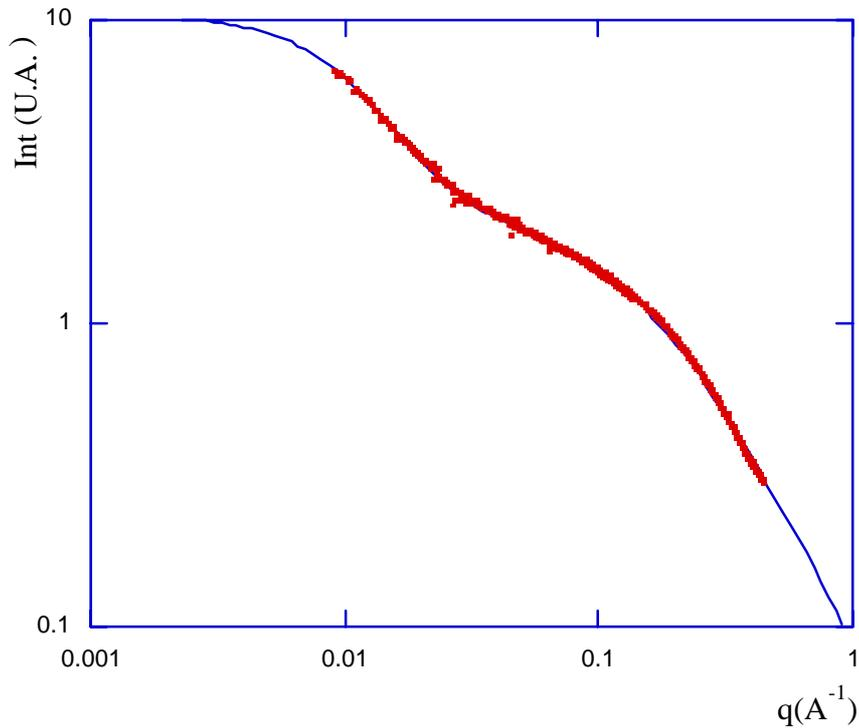
Fig. 1 : Scattering of the PAASr200 at E=15.8KeV. The line is the fit to the sum of a OZ and a DB equations.
