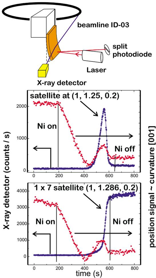
Fig. 1. Schematic of the curvature measurement at ID-03 by an optical deflection technique. Simultaneously taken curvature data –right axes – and X-ray diffraction data – left axes – during the growth of the first monolayer Ni on W(110). See text for details.
