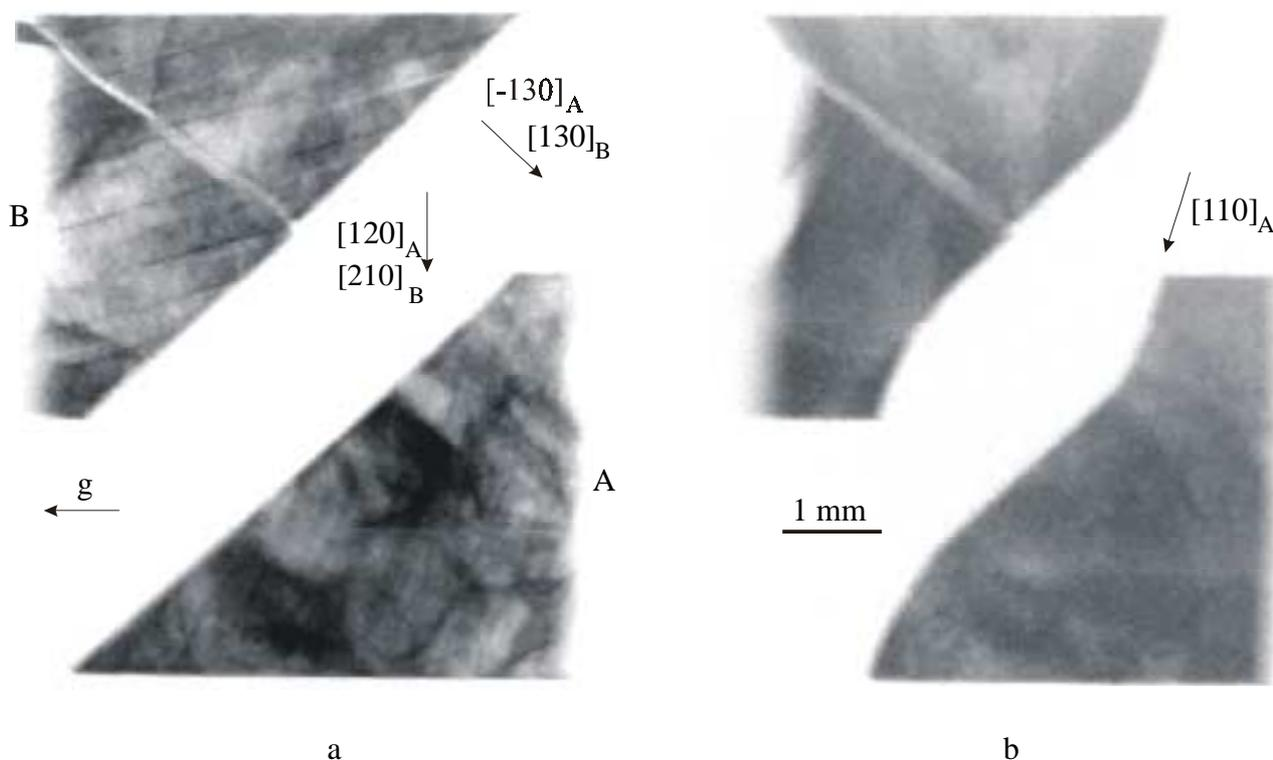
Fig.1 *In situ* topographs of a  $\Sigma 5$  bicrystal before annealing (a) and after 75 min at 965°C (b).
