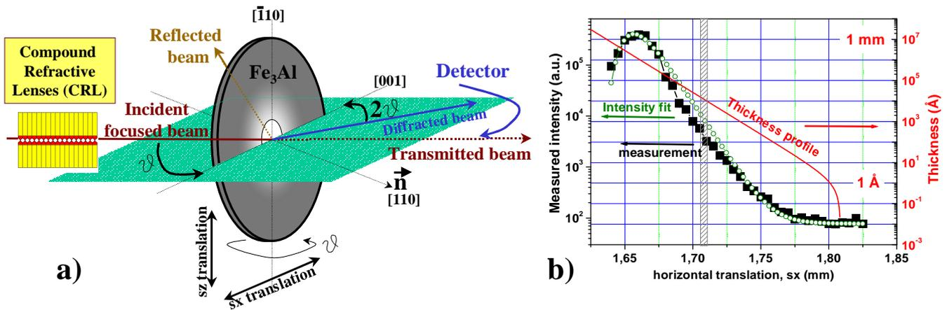
**Figure 1:** a) sample geometry for the diffraction experiment; b) hole profile obtained by scanning the sample position at the lattice peak (002) position. The edge position is  $s_x=1.8$  mm. The hatched area (around  $s_x=1.705$  mm) indicates the measured position at the rim of the hole.
