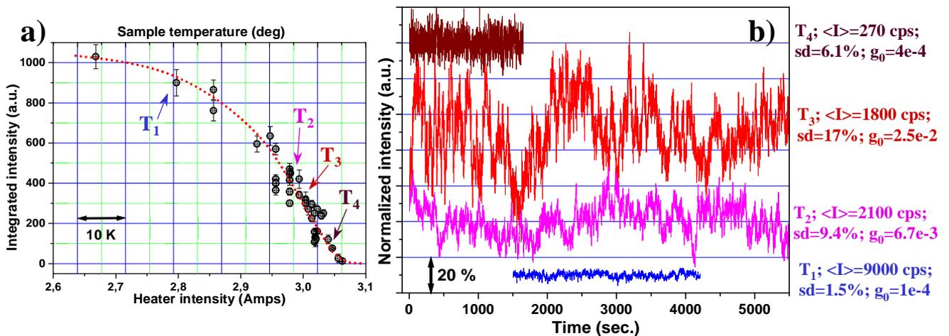
**Figure 2:** a) integrated intensity of the superstructure (113) peak measured at different temperatures near  $T_c$ . The dotted line is just a guide for the eye. For the temperatures denoted by  $T_1$  to  $T_4$ , timescans are shown in figure b), using the same relative scale. The average intensity was normalized to 1. The values of the average intensity  $\langle I \rangle$  in counts/s, standard deviation (sd), and  $g^{(2)}(\tau \rightarrow 0)-1$  (denoted by  $g_0$ ) are shown.
