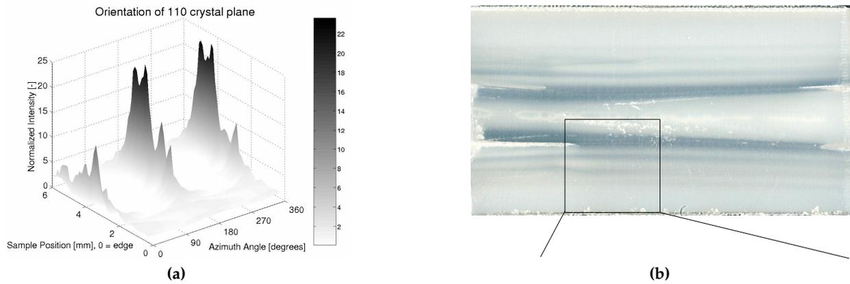
**Figure 2:** (a) 110 crystal-orientation over a sample width of 6 [mm], from edge to center of the sample. The peaks between 4 and 5 [mm] of the edge correspond to a region with highly oriented structures in the sample. (b) Scan from a sample, produced with the MPR with a high piston speed, i.e. a high shear rate (sample thickness  $\pm 2$  [mm]). Dark regions are in reality transparent. Scan is made with dark background for a better contrast.
