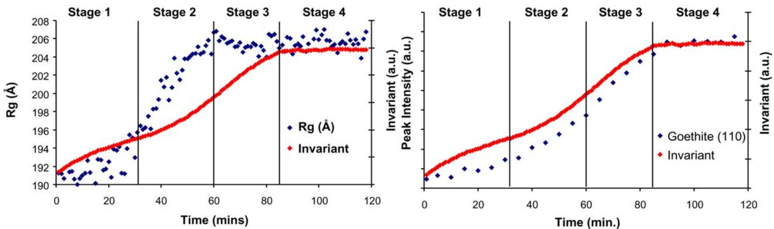
Figure 2 (a)  $R_g$  and SAXS invariant and (b) goethite (110) Bragg peak intensity and SAXS invariant as a function of time for the crystallisation of goethite from phosphate doped ferrihydrite. Note that the crystallisation process can be divided into 4 stages.
