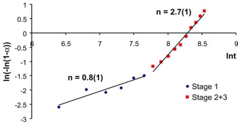
Figure 3. Avrami plot of the geothite (110) Bragg peak intensity. Avrami exponent for stage 1 and stages 2+3 are marked.
