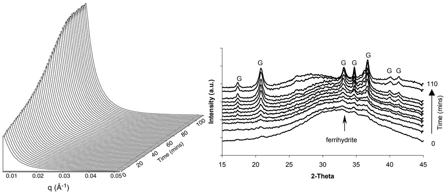
Figure 1. Time-resolved (a) SAXS (b) WAXS plots for the crystallisation of goethite from phosphate doped ferrihydrite. Note the broad ferrihydrite peak in the WAXS data at  $T=0$ . This rapidly decreases with time as peaks for goethite (G) grow.
