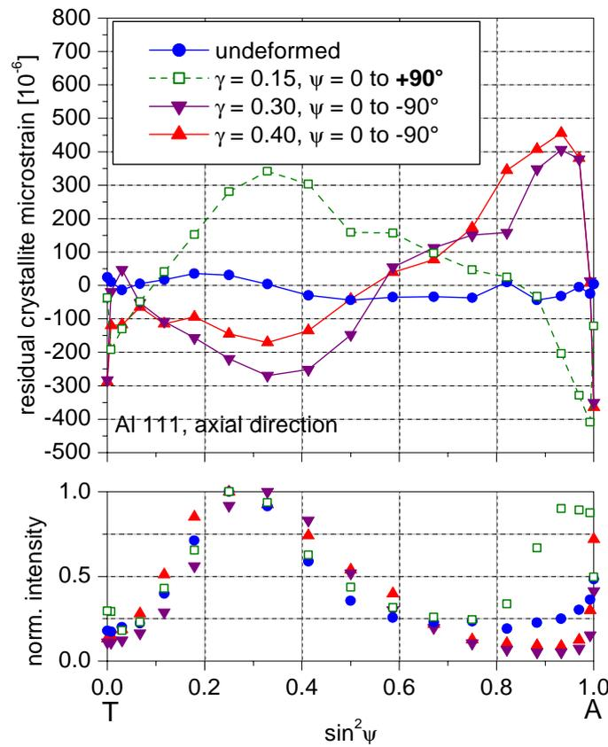
**Figure 2:** Crystallite microstrains measured on the Al 111 reflection in tubular AlMg3 torsion samples in different deformations. Note the different  $\psi$  range of  $0^\circ$  to  $+90^\circ$  for the deformation  $\gamma = 0.15$ . Average error:  $\pm 15 \times 10^{-6}$ .
