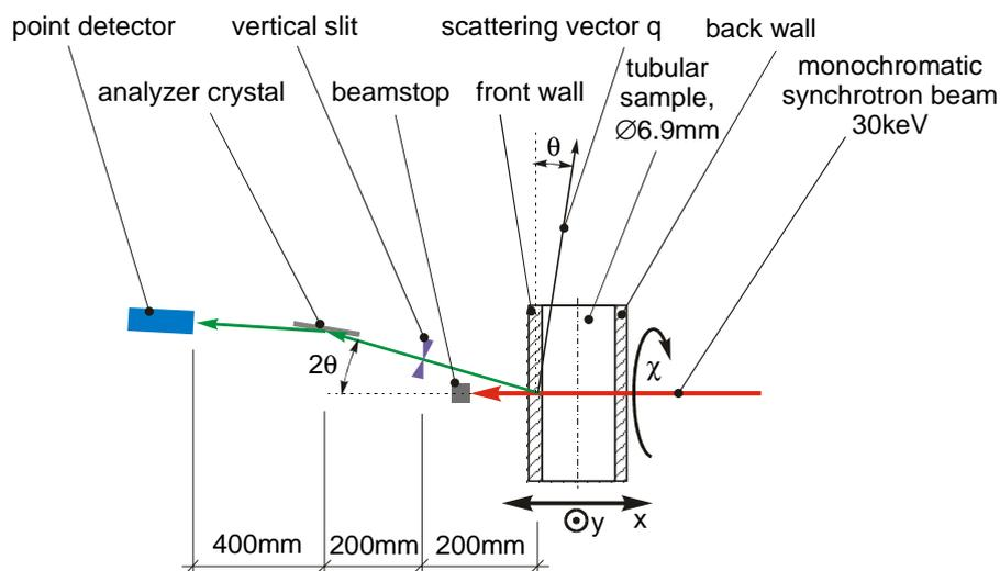
**Figure 1:** Experimental setup for angle dispersive technique, using analyzer crystal and point detector
