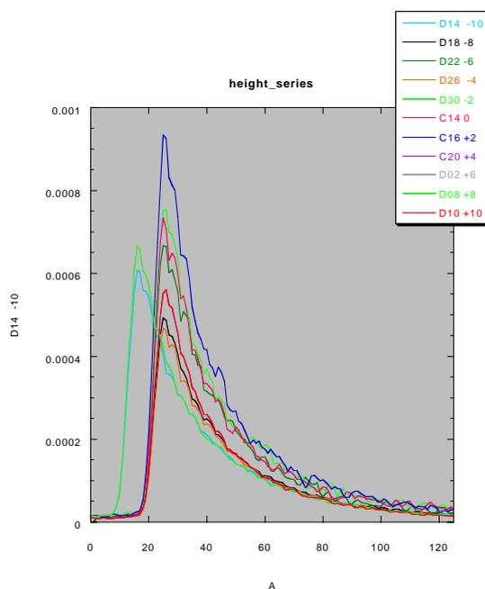
Fig. 1 Preliminary *in situ* SAXS profiles obtained for soot formation at different flame heights in a methane flame using a purpose-built gas slot burner on BM26B.
