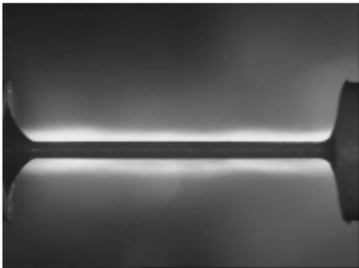
*Fig. 1 Human bone specimens in the microtensile testing system.*
