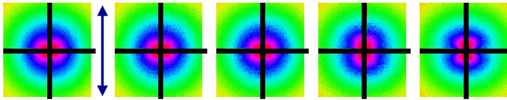
Figure 1. USAXS speckle patterns from carbon black N330 dispersed in uncross-linked EPR. From left to right: before stretching, stretched in the direction of the arrow at  $\epsilon=0.02$ ,  $\epsilon=0.07$ ,  $\epsilon=0.27$ ,  $\epsilon=0.53$ . The distance between the centre and any side of the square is equal to 50 pixels (corresponding to  $4 \times 10^{-2} \text{ nm}^{-1}$ ).
