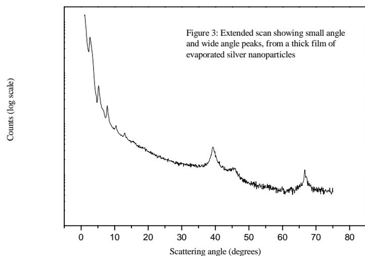
Extended measurements of a thick film of the dodecanethiol capped silver particles were made, to cover both the small angle and the wide angle scattering (figure 3). The wide angle features were interpreted using the Debye-Scherrer formula to determine the broadening of the peak, due to the crystal size. This gave a value of 5.5nm again indicating a lack of long-range order in the assembly process.
