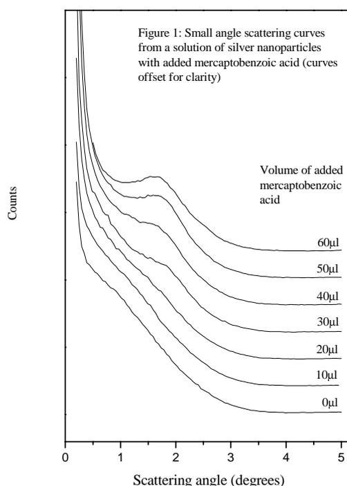
mercaptobenzoic acid is added, the clusters start to aggregate together forming a scattering object of interacting particles. This causes a distinct peak to appear at a scattering angle of  $\sim 1.67^\circ$ , that can be interpreted as the separation of the particles in a distorted close packed structure. This yields a separation of approximately 6.7nm using Hosemann's cubic paracrystal model. These results are consistent for the interaction being driven by the mercaptobenzoic acid.
