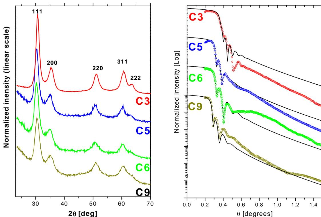
**Fig. 1.** Left: Recorded x-ray diffraction patterns of samples C3-C9.  $\lambda=1.2398 \text{ \AA}$ , angle of incidence:  $0.7^\circ$ . Right: Reflectivities of samples C3-C9 (points) as compared with simulated curves (solid lines).  $C_n$  symbols refer to number of carbon atoms in the dithiol spacer molecules.
