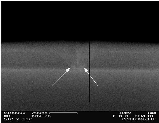
**Fig. 2** SEM picture of overgrowth with InGaP
