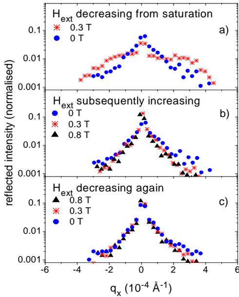
Figure 1 Off-specular SMR scans of a MgO(001)/[<sup>57</sup>Fe(26Å)/Cr(13Å)]<sub>20</sub> ML in external fields parallel to an easy axis. In a field of 0.3 T decreasing from saturation to remanence, the in-plane AF domain size is about  $\xi = 0.5 \mu\text{m}$ , which increases to  $\xi = 2.6 \mu\text{m}$  in remanence. No further change is observed on increasing or decreasing the field without saturating the ML again.
