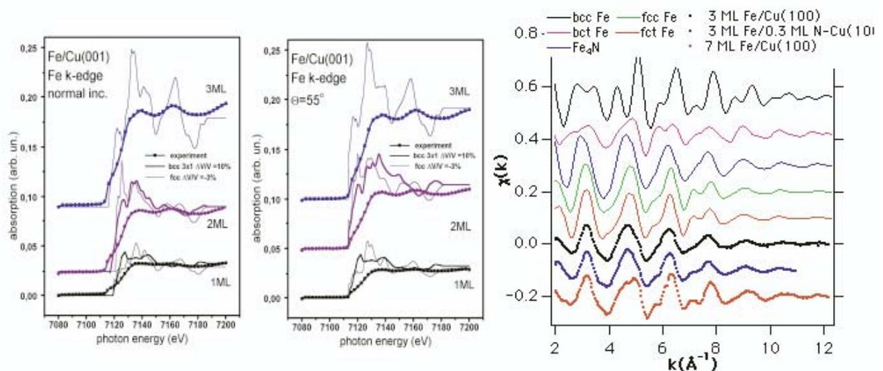
**Fig. 2.** Comparison between experimental data and multi-shell model data of the near edge and extended absorption region. See labels in the figures for details about the model structures.
