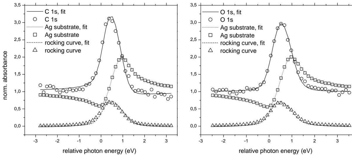
Figure 1: NIXSW measurements and corresponding fit curves for a relaxed (left) and compressed (right) monolayer structure of NTCDA on Ag(111) at room temperature. The relative absorption versus photon energy curves (relative to the Bragg energy of 2.625 keV) are shown together with the rocking curves of the Ag(111) Bragg reflection and the substrate curve derived from the photoelectron background.
