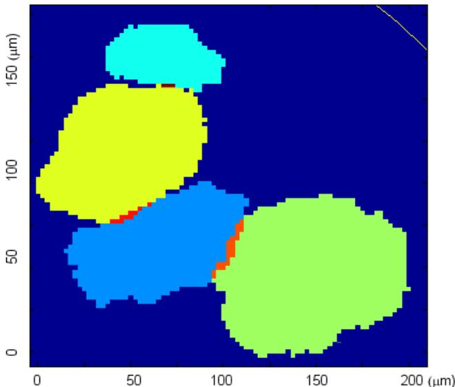
**Fig. 4.** Independent reconstruction of 4 neighbouring grains marked by different colours. Regions of overlap between the grains are marked by red. The surface of the polycrystal is indicated by a solid yellow curve.
