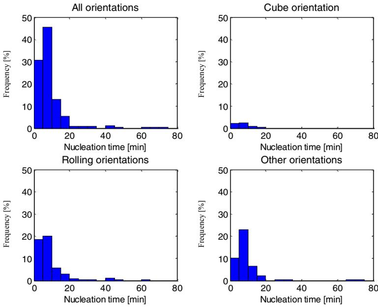
**Fig. 2.** Histograms of nucleation times (in minutes). The frequencies based on all grains is shown in the upper, left corner. Next, the grains are sorted into three texture groups; cube, rolling and other. The respective fractional frequencies are shown. The result of a Kolmogorov-Smirnov test is that the 4 distributions are identical within error.
