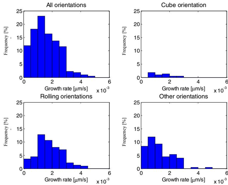
**Fig. 3.** Histograms of initial growth rates in  $\mu\text{m/s}$  (for  $t = 600\text{s}$ ). The frequencies based on all grains is shown in the upper, left corner. Next, the grains are sorted into three texture groups; cube, rolling and other. The respective fractional frequencies are shown. Grains having cube and rolling orientations are seen on average to have a higher initial growth rate than grains with random orientations.
