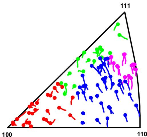
**Fig. 1.** Stereographic triangles showing the rotation of the tensile axis of individual bulk grains during tensile deformation measured in three experiments on different fcc metals. The circles mark the final orientation of the grains[14].
