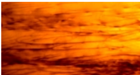
Figure 1: Dislocations in a prismatic diffraction plane observed in a 1mm thick ice thin section (monochromatic beam, \lambda=0.69 \text{ \AA} ).
