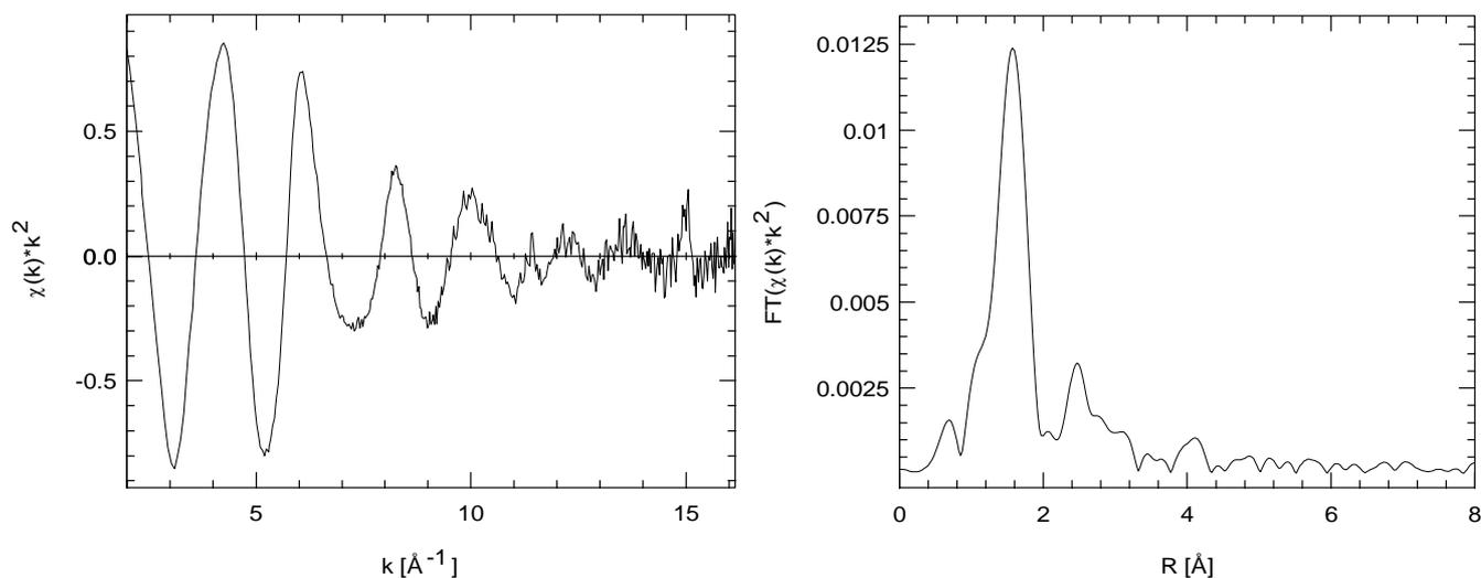
**Figure 1:** The Sn EXAFS and its Fourier transform from a single XAS scan of 0.25%Pt-1.25%Sn/Mg(Al)O used in propane dehydrogenation (not exposed to air).
