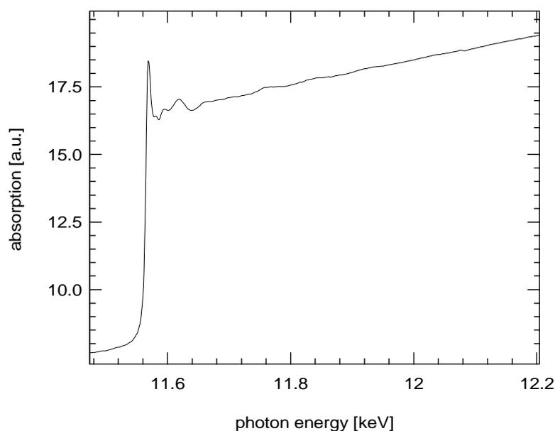
**Figure 2:** The Pt L<sub>III</sub> XAS profile (single scan) of 0.25%Pt-1.25%Sn/Mg(Al)O used in propane dehydrogenation (not exposed to air).
