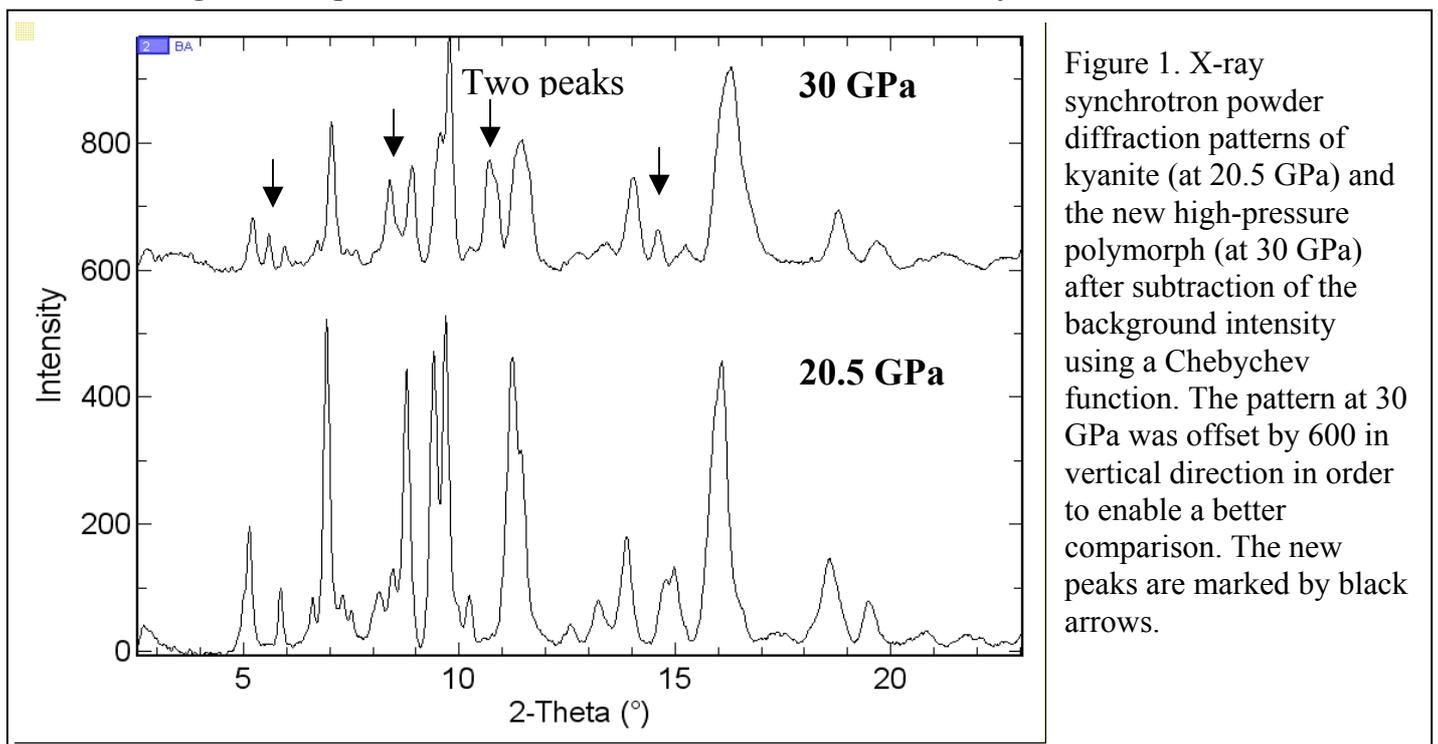
Figure 1. X-ray synchrotron powder diffraction patterns of kyanite (at 20.5 GPa) and the new high-pressure polymorph (at 30 GPa) after subtraction of the background intensity using a Chebychev function. The pattern at 30 GPa was offset by 600 in vertical direction in order to enable a better comparison. The new peaks are marked by black arrows.
