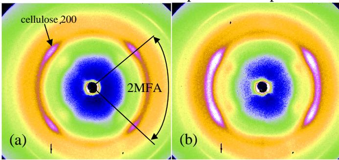
Figure 1: WAXS patterns collected during a stress-strain experiment on a slice of *Picea abies*. The frames left (a) and right (b) were taken at the beginning and at the end of the tensile experiment, respectively. The mutual position of the equivalent cellulose 200 reflectionse is proportional to the magnitude of 2xMFA. During the experiment, MFA decreased from 45 to 30 degrees.
