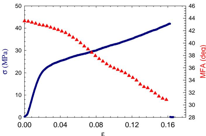
Figure 2: In-situ synchrotron experiment on a wet foil of *Picea abies* - a typical stress-strain curve (blue) and a strain dependence of MFA (red triangles). The sample was strained with a strain rate of 0.025 mm/s and the frames were collected for 4 seconds. The nearly linear experimental dependence of MFA on strain is in a very good agreement with the relationship  $MFA(\epsilon) = MFA(0) - \cotg[MFA(0)] \epsilon$ .
